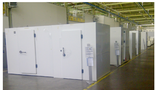
Set up of cold rooms from 19 different suppliers for energy efficiency tests by TÜV Süd
